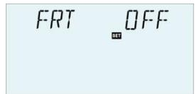
▶ Press “↑”, “↓” button, to activate this function, “FRT ON” displays on the screen
