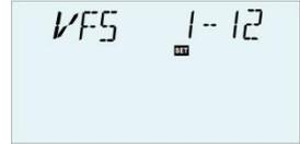
▶ Press “↑”, “↓” button, to adjust the measurement range of flow meter
